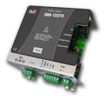
The battery charger, SBB12070 is specially designed for emergency generators and diesel engine fire pump starter batteries. Permanently connected to the battery, it constantly monitors the condition of the batteries and always keeps them at maximum capacity. The SBB12070 battery chargers remain on during the engine starting process.
